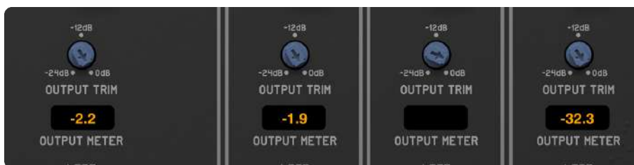
Figure 55. Trim knobs for direct outputs
